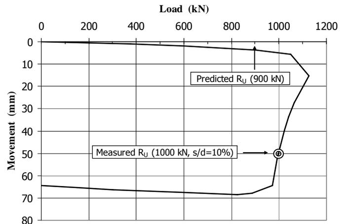
Figure 6. SLT: predicted and measured capacity
