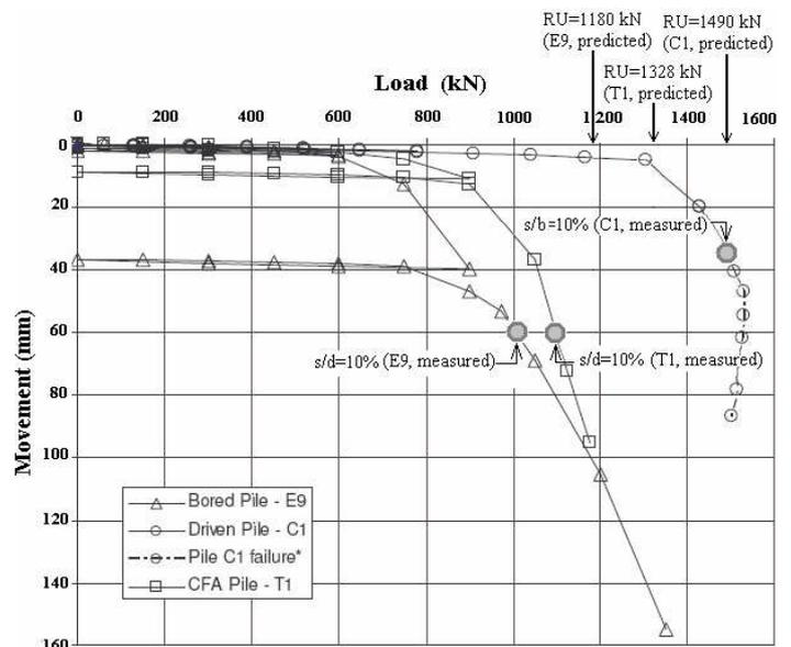
Figure 9. SLT: predicted and measured capacities
