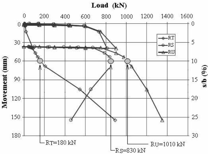
Figure 10. Pile E9 (measured  $R_S$ ,  $R_T$  and  $R_U$ )
