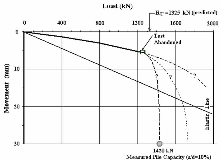
Figure 3. SLT: predicted and measured capacity
